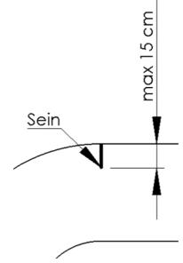
Figure 4: Hindering wall (top view)
